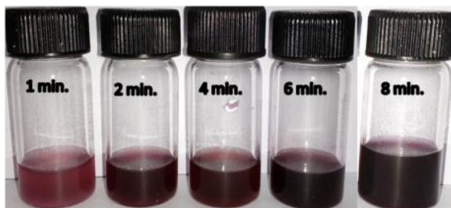
Fig 10 : Picture showing AuNP colour changing pattern. 0.1% gum solution with 1mM concentration of H Au Cl 4
