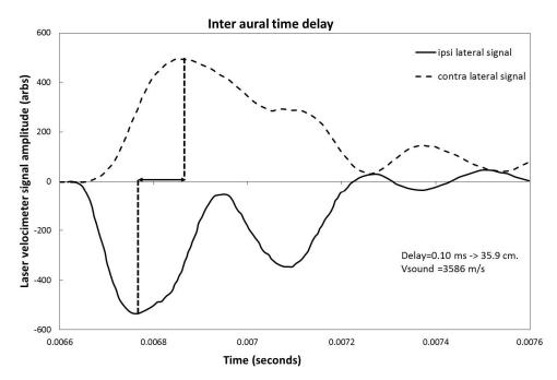
Figure 5. Measurement by laser velocimeter of the inter-aural time response of the round window driven by a 220  $\mu$ s square pulse. For better visualization, the ipsilateral signal (full line) has been inverted with respect to the contralateral signal (dashed line).
