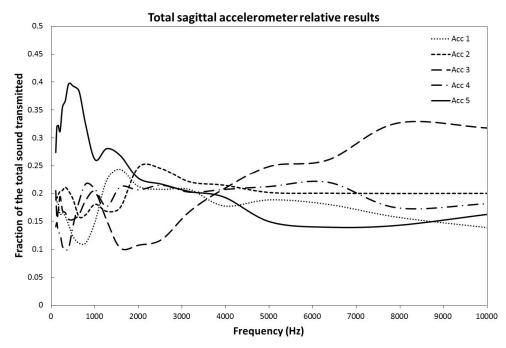
**Figure 4.** Relative fraction of the signal transmitted across the sagittal line by each of the five accelerometers set along it as a function of the implant signal frequency. The results have been averaged over all orientations of the BAHA<sup>TM</sup> implants about the Frankfort plane.
