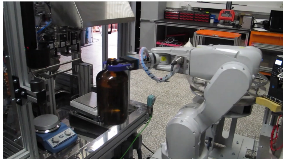
Figure 1. Flexible manufacturing system for solution preparation: robot carrying a bottle.
