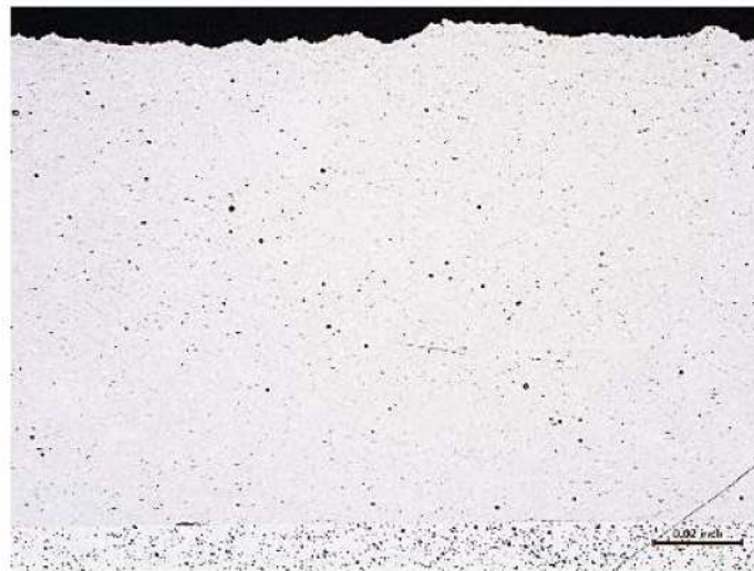
Figure 7. Micrograph depicting typical microstructure observed on aluminium 2024 cold-sprayed coating on aluminium 2024 substrate. As-etched; At 25\times .
