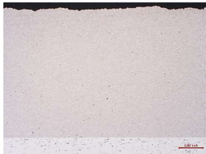
Figure 8. Micrograph depicting typical microstructure observed on aluminium 7075 cold-sprayed coating on aluminium 7075 substrate. As-etched; at 25\times .
