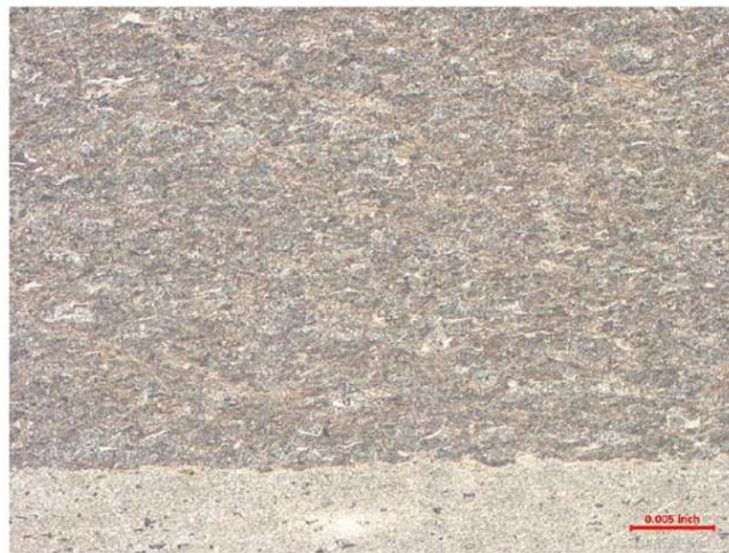
Figure 9. Micrograph depicting the typical microstructure observed on Al-2024 cold-sprayed coating on Al-2024 substrate. As-etched; at 100 \times .
