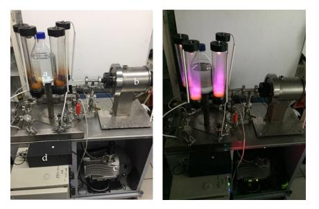
**Figure 1.** Plasmothrone (without cover) used in this study. (**a**) Lamps, (**b**) pulse generator, (**c**) vacuum pump, and (**d**) power supply [19].
