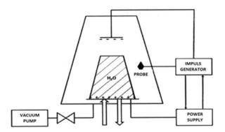
Figure 2. Scheme of the glow plasma (GP) generator and the mode of treating water with it [18].
