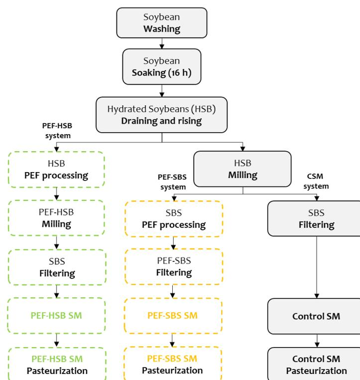
**Figure 1.** General soymilk (SM) preparation procedure with the application of low-intensity pulsed electric fields (PEFs) in hydrated soybeans (HSB) and soybean slurry (SBS).
