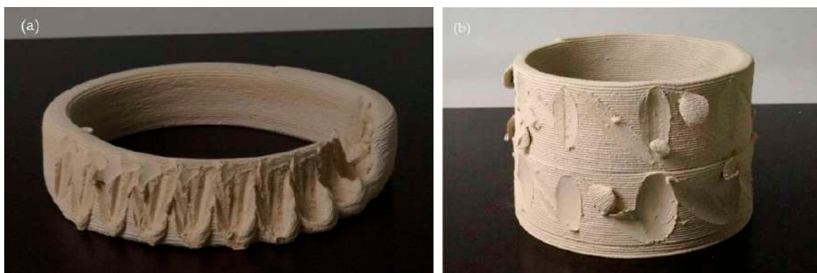
Figure 5. Comparison blurring artefact with the nozzle (a) and with the cutting tool (b).
