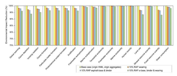
**Figure 5.** LCA results for the studied road using  $\leq$ 10% RAP content in pavement courses vs. baseline.
