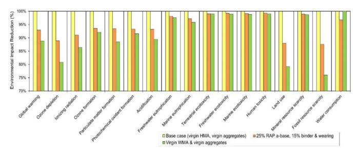
**Figure 7.** LCA results for the studied road using  $10\% \le 25\%$  RAP content vs. baseline.
