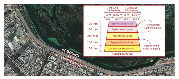
Figure 2. Case-study asphalt pavement section.
