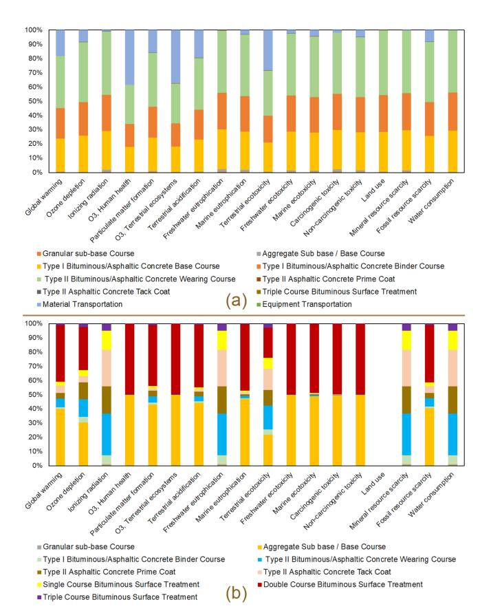
**Figure 4.** LCA results for the studied road in the baseline scenario using virgin materials for all lifecycle stages: (a) raw material extraction, processing, equipment and material transport to construction site, including M&R material; (b) construction and M&R.
