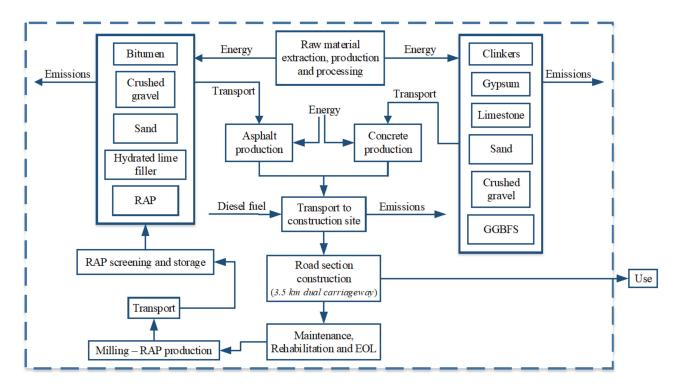
Figure 3. System boundary considered for the studied pavement section.
