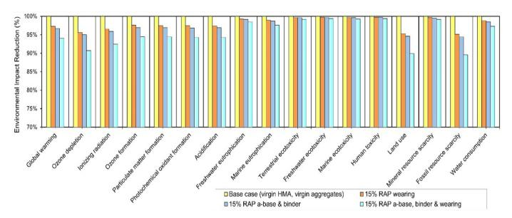
**Figure 6.** LCA results for the studied road using  $\leq$ 15% RAP content in pavement courses vs. baseline.
