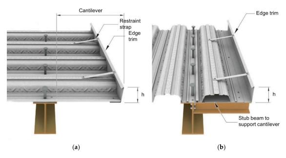
**Figure 1.** Typical edge configurations: (a) perpendicular orientation of the steel decking; and (b) parallel orientation of the steel decking [1].
