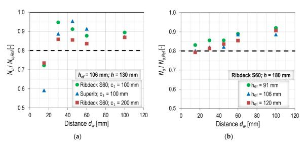
**Figure 8.** Numerical results of Series 1 for: (a) the embedment depth  $h_{ef}$  = 106 mm; and (b) the overall member thickness h = 180 mm.
