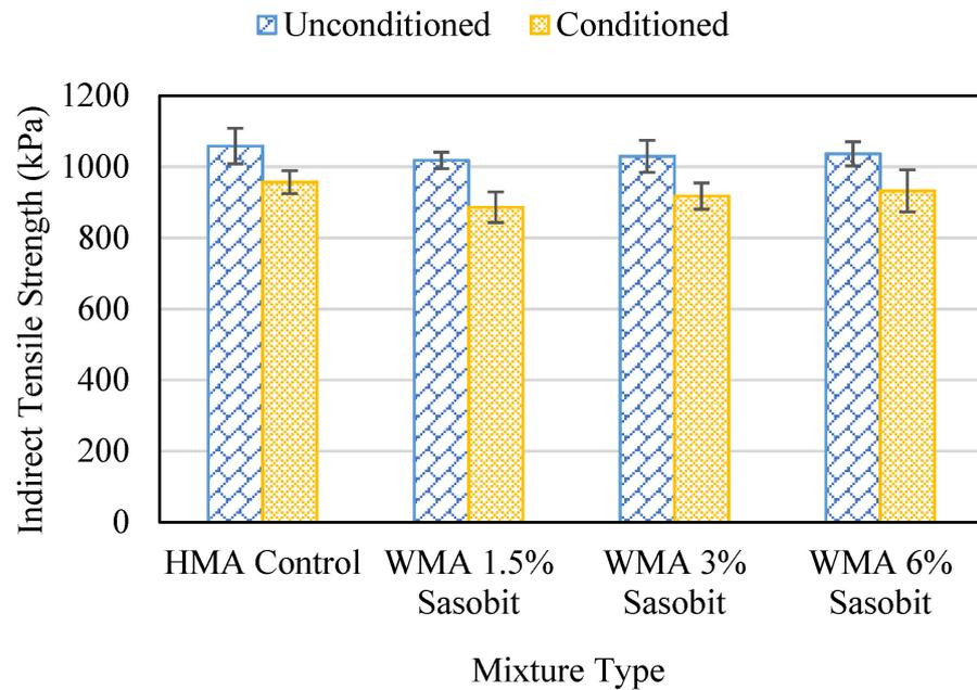
Figure 6. The results of indirect tensile strength of different asphalt mixtures.
