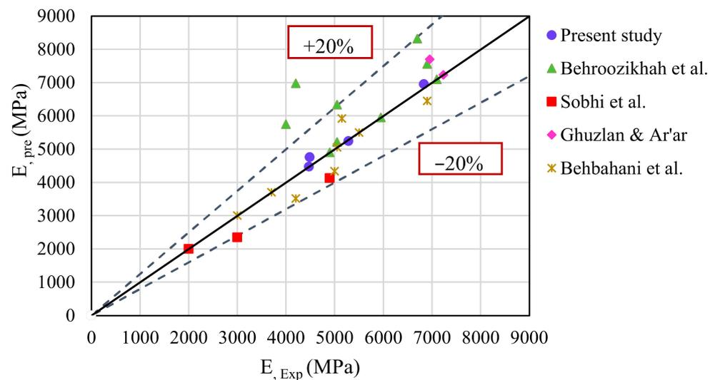
**Figure 5.** Comparison of the resilient modulus between the proposed model and the laboratory results of other researchers.
