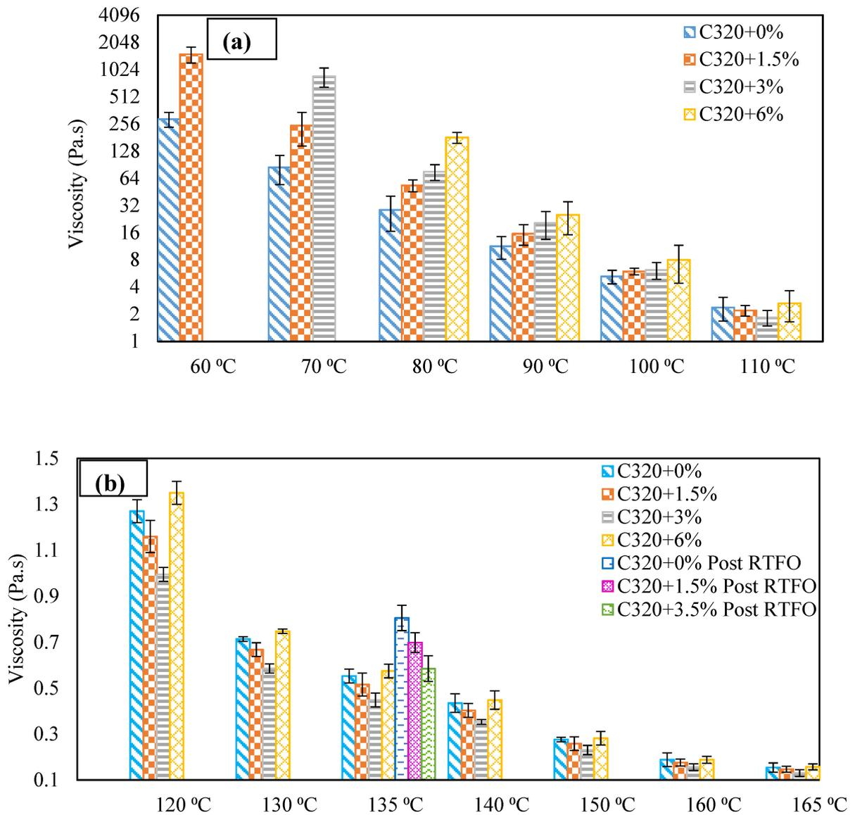
**Figure 3.** Viscosity results at different temperatures for C320 bitumen mixed with Sasobit: (a) viscosity at 60 °C to 110 °C; (b) viscosity at 120 °C to 165 °C.
