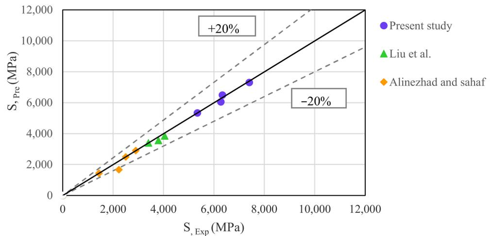
**Figure 14.** Comparison of the r flexural stiffness results between the proposed model and the laboratory results of other researchers.
