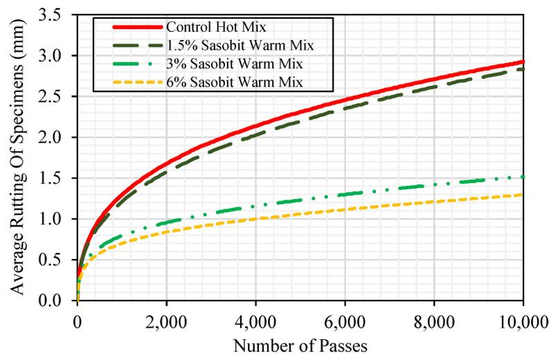
**Figure 15.** Comparison of wheel tracking results for HMA and WMA.
