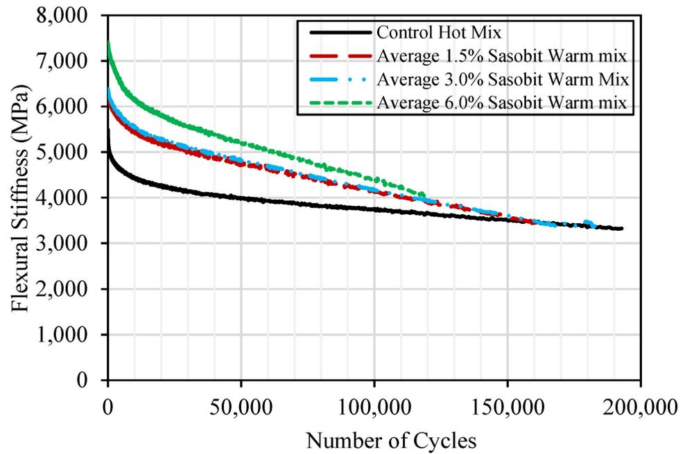
Figure 12. Comparison of average fatigue resistance for HMA and WMA.
