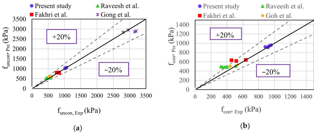
**Figure 8.** Comparison of the tensile strength results between the proposed model and the laboratory results of other researchers: (a) conditioned samples; (b) unconditioned samples.
