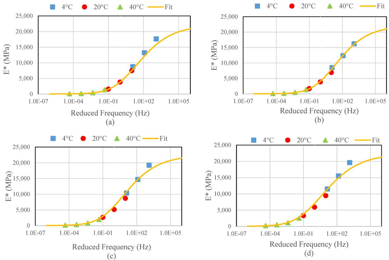
**Figure 9.** Master curves results: (a) HMA samples; (b) WMA with 1.5% Sasobit; (c) WMA with 3% Sasobit; (d) WMA with 6% Sasobit.
