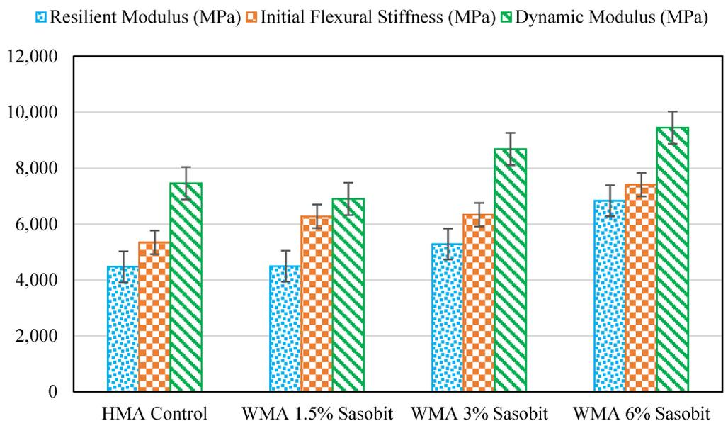
Figure 13. Comparison moduli at 20 °C and 10 Hz loading rate.
