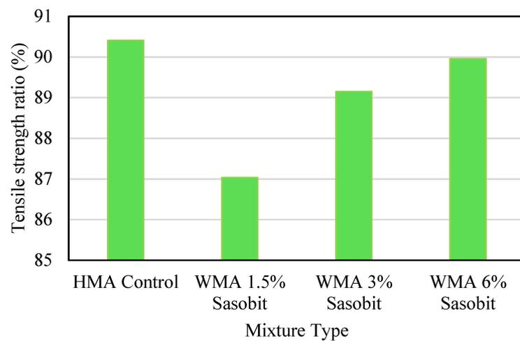
Figure 7. TSR values of different asphalt mixtures.
