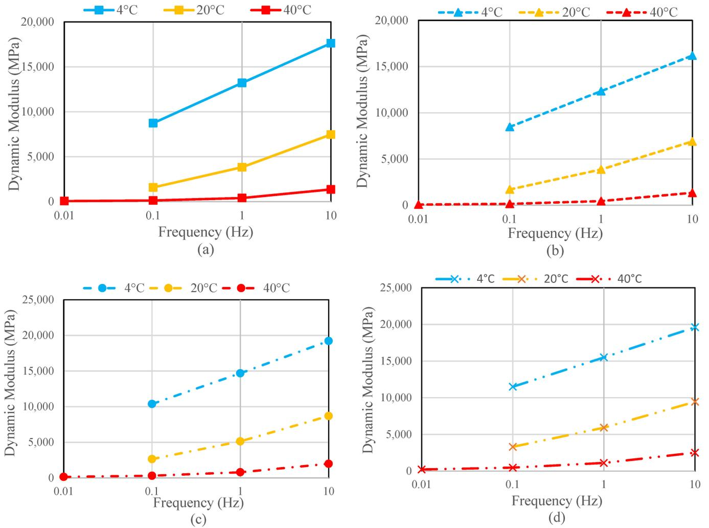
**Figure 10.** Dynamic modulus results: (a) HMA samples; (b) WMA with 1.5% Sasobit; (c) WMA with 3% Sasobit; (d) WMA with 6% Sasobit.
