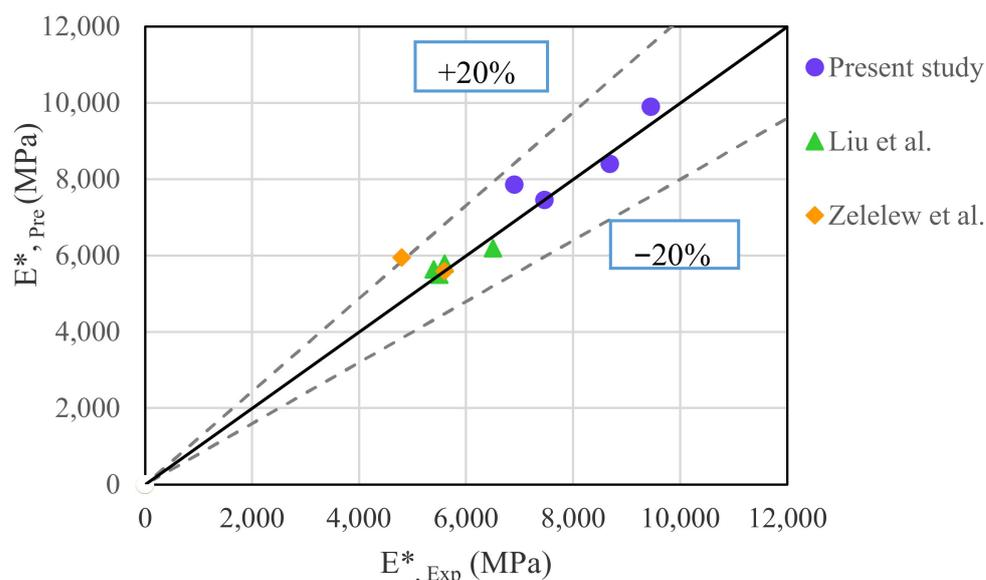
**Figure 11.** Comparison of the dynamic module results between the proposed model and the laboratory results of other researchers.
