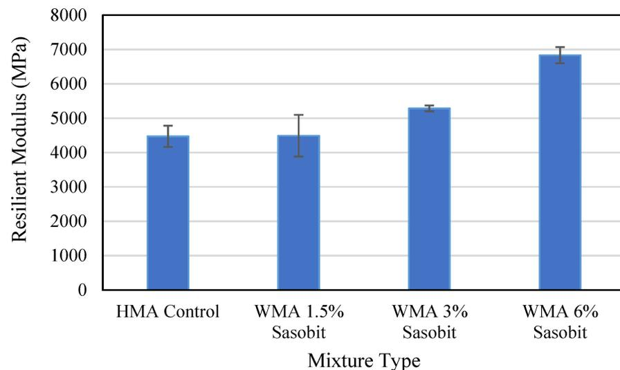
**Figure 4.** Resilient modulus test results of different asphalt mixtures.
