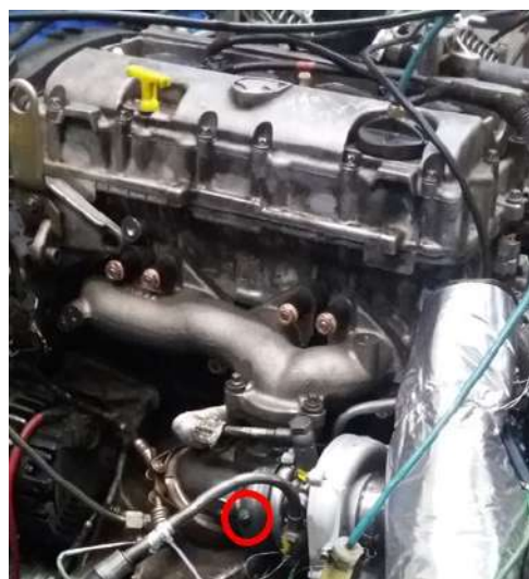
Figure 5. Location of a thermocouple on the turbocharger housing.
