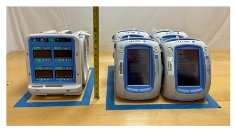
**Figure 9.** Photograph of blue tapped footprints of the RX-4 (left) and four VAC Ulta devices with a tape measure between the two measuring the height of each device (RX4 = 11.5 cm (left) and the Vac Ulta = 10.5 cms (right)).
