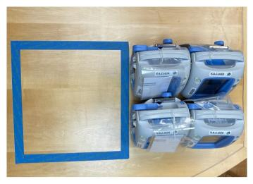
**Figure 8.** Photograph of a blue tapped border representing the footprint of four VAC Ulta units. Immediately adjacent are the four VAC Ulta devices. The length and width of the four VAC Ulta devices measure  $15.75 \text{ cm} \times 17 \text{ cm}$ .
