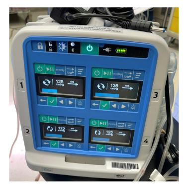
**Figure 7.** Photographof the RX-4 device with all four channels set at -125 mmHg for NPWT delivery.
