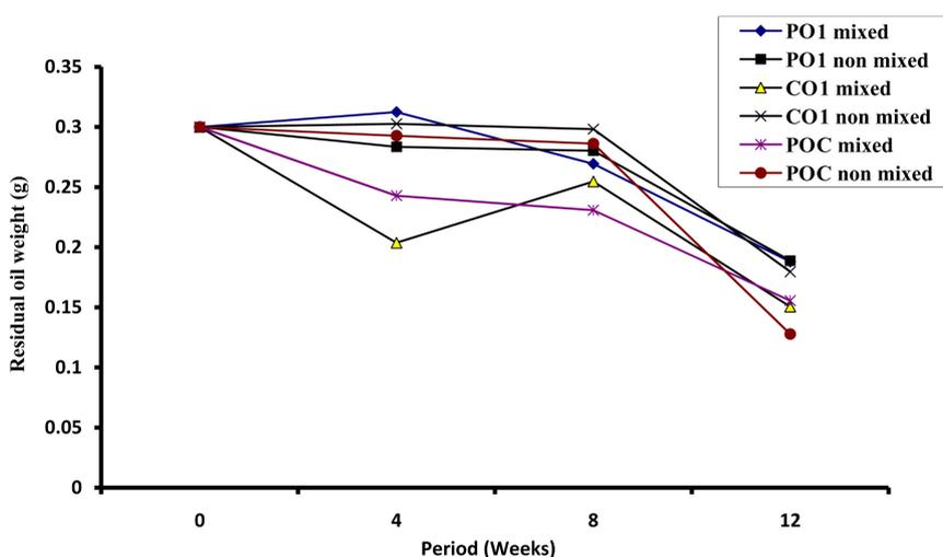
**Figure 13.** Total recoverable residual oil in sterile palm kernel oil contaminated sample with and without mixing.
