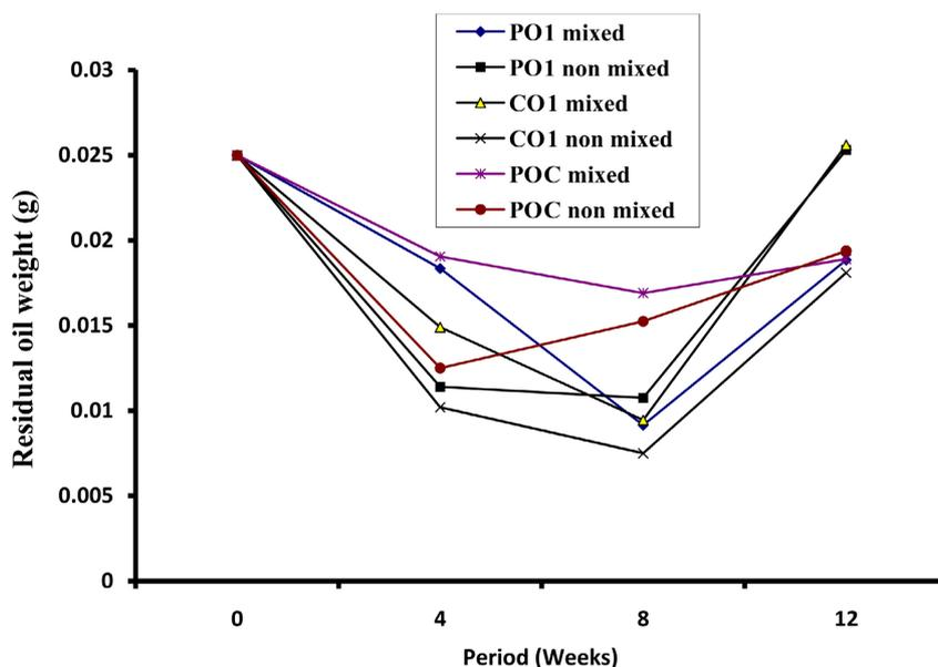
**Figure 9.** Total recoverable residual oil in sterile oil mill sample with and without mixing.
