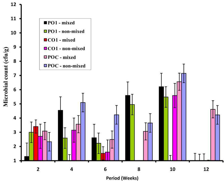
**Figure 2.** Total viable microbial count in non-sterile soil samples from oil mill with and without mixing.
