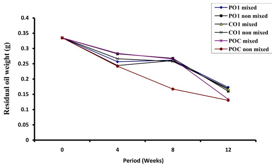
**Figure 15.** Total recoverable residual oil in sterile palm oil contaminated sample with and without mixing.
