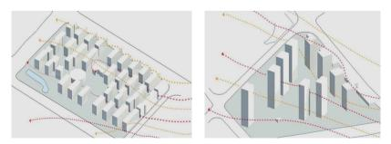
**Figure 3.** Blocks E (left) and H (right): heights, densities, and indicative summer wind flow. The analysis suggests ways of wind flow in between high-rise urban blocks vs. opportunities for cross ventilation in the low-rise typologies.
