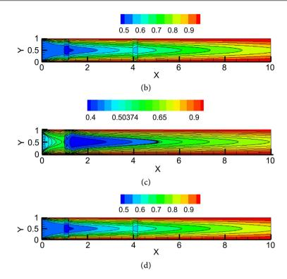
**Figure 2.** The normalized temperature profile plotted for Re = 100 using statistical technique (a) for single strainer, (b) for a double strainers and quantum technique (FDM) for (c) for a single strainer, (d) for double strainers.
