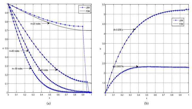
**Figure 1.** (a) A Stability study of case (1) for various Number of Nodes/Lattices and (b) A Study of case (2) for various time step using Statistical Approach (LBM) & Quantum Approach (FDM).
