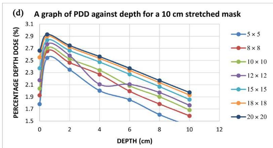
**Figure 3.** (a) PDD against depth without mask at different field sizes; (b) PDD against depth with an unstretched mask at different field sizes; (c) PDD against depth with 5 cm stretched mask at different field sizes; (d) PDD against depth with 10 cm stretched mask at different field sizes.
