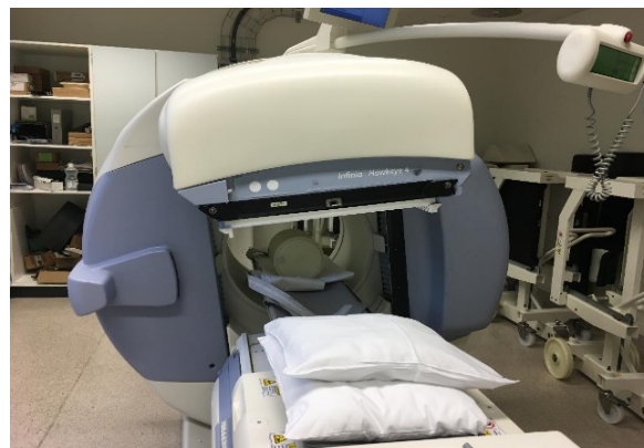
Figure 5. Cross calibration phantom set up on Infinia Hawkeye 4 SPECT/CT system.
