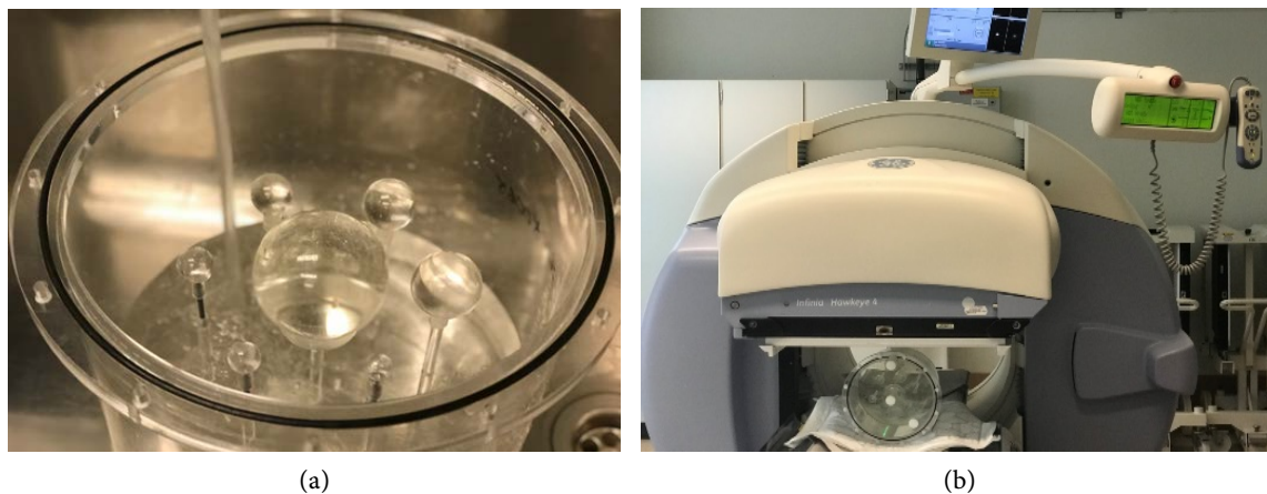
Figure 6. (a) Filling background with water; (b) 3D sensitivity test acquisition.
