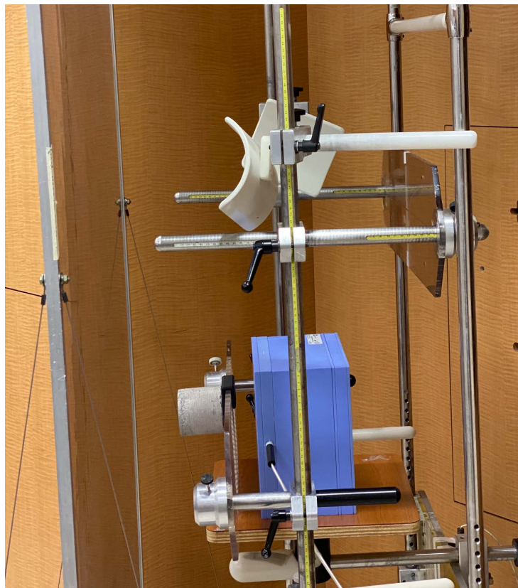
Figure 2. The ion chamber setup used for phantom measurements.
