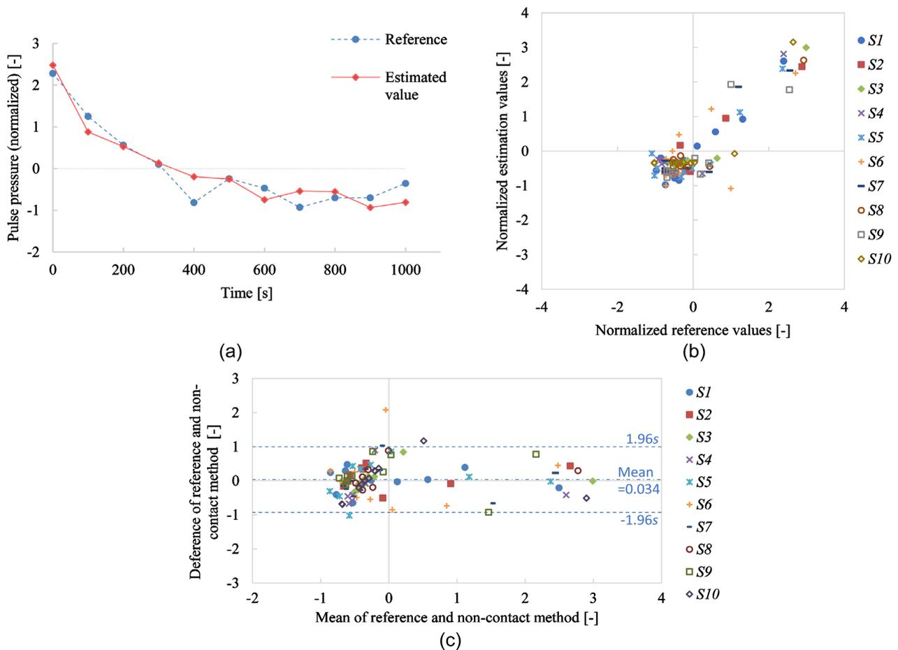
**Figure 4.** Results of Experiment 1. (a) Sample of the results of the change in pulse pressure induced by the ergometer task in Experiment 1 (subject  $S_1$ ). (b) Comparison of the two results measured by the contact method as a reference and the estimation results based on noncontact measurement ( $r = 0.884$ ). (c) Bland-Altman plot for all subjects (mean = 0.034, upper coefficient limit = 10.998, lower coefficient limit = -0.930).
