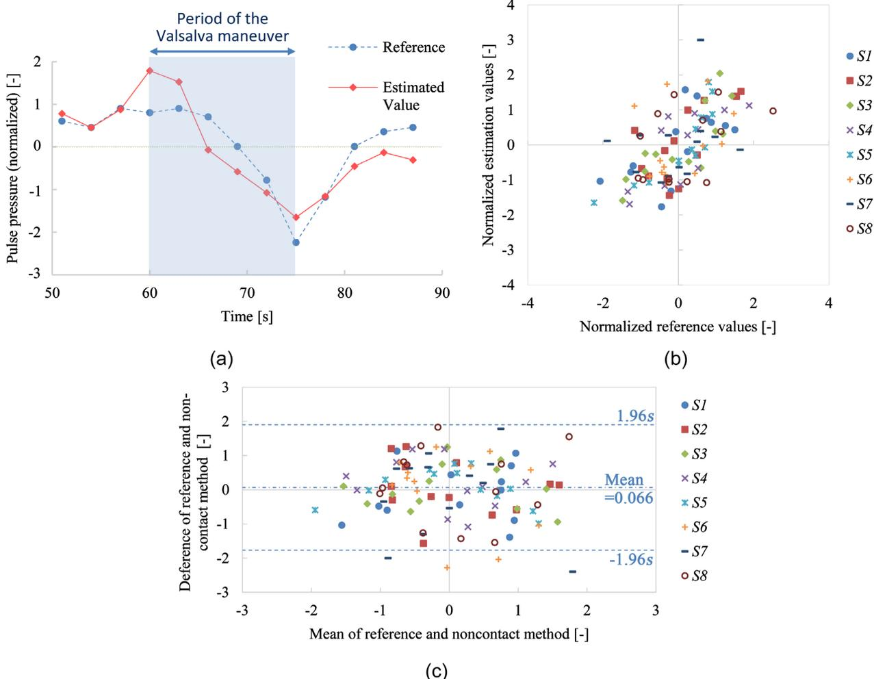
**Figure 5.** Results of Experiment 2. (a) Sample of the results of the change in pulse pressure induced by the Valsalva maneuver in Experiment 2 (subject  $S_1$ ). (b) Comparison of the two results measured by the contact method as a reference and the estimation results based on noncontact measurement ( $r = 0.575$ ). (c) Bland-Altman plots for all subjects (mean = 0.066, upper coefficient limit = 1.902, lower coefficient limit = -1.770).
