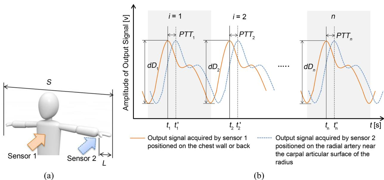
**Figure 1.** (a) Measurement points and coordination. (b) Image of acquired waveform and parameters which assigning values to estimation equation.
