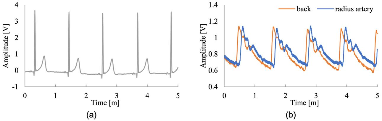
**Figure 3.** Sample signals measured by contact and noncontact methods. (a) Sample ECG signal as reference. (b) Sample signals of the noncontact method using microwave radar (upper part acquired at the back and lower part acquired at the radius).
