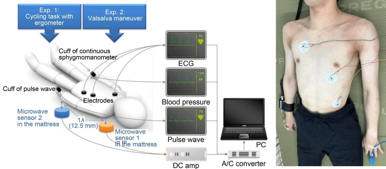
**Figure 2.** Experimental setting and block diagram of the experiments. (a) Schematic block diagram of the experimental setting. (b) Photograph showing Experiment 2.
