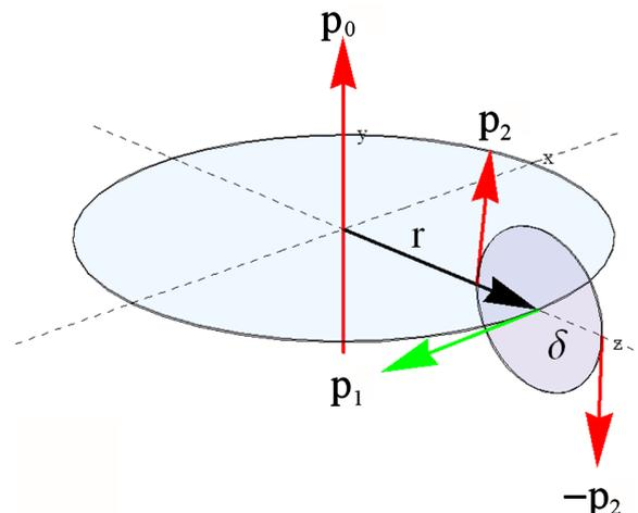
**Figure 7.** Momentum density  $p_0$  (red) induces C-field circulation at position  $\mathbf{r}$ . The C-field circulation at  $\mathbf{r}$  yields momentum density  $p_1$  (green) orthogonal to  $p_0$ . Momentum  $p_1$  induces the C-field at distance  $\delta$  from  $p_1$ . This induced C-field yields momentum density  $p_2$  (red) with components parallel and anti-parallel to  $p_0$ .
