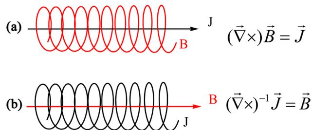
**Figure 3.** (a) Linear charge current density  $\mathbf{J}$  induces magnetic  $\mathbf{B}$  field circulation; (b) Solenoidal current induces axial magnetic field  $\mathbf{B}$ .
