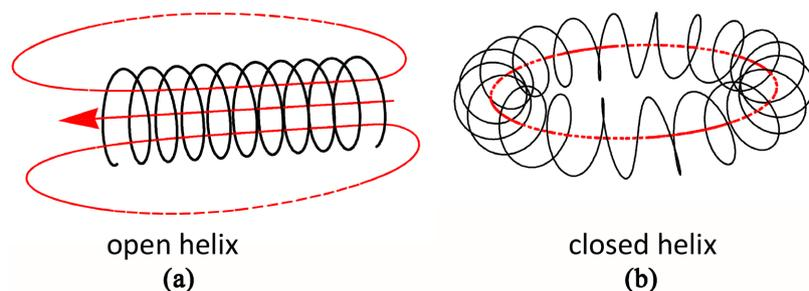
**Figure 5.** (a) The field induced by helical current in an open helix resides both on the helical axis and is distributed over space surrounding the helix; (b) Magnetic field induced by the same current in a closed helix is constrained to reside on the (closed) helical axis; total induced field is assumed to be the same, thus the closed-helix-induced energy-density is assumed greater than the axial density of the open helix.
