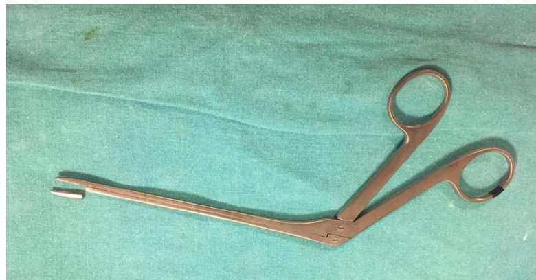
Figure 4. Disc rongeur and broken tip (20 × 5 mm) removed from the intervertebral space (black arrow).
