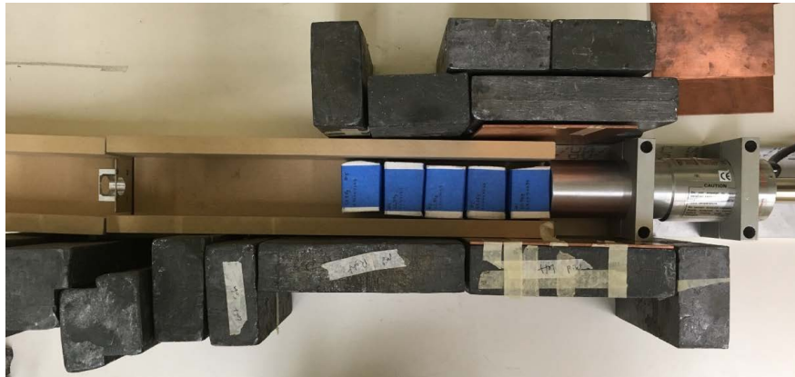
Figure 2. Top view of the Experimental Setup. Left to right: source holder, trough with organic blocks, HPGe detector.
