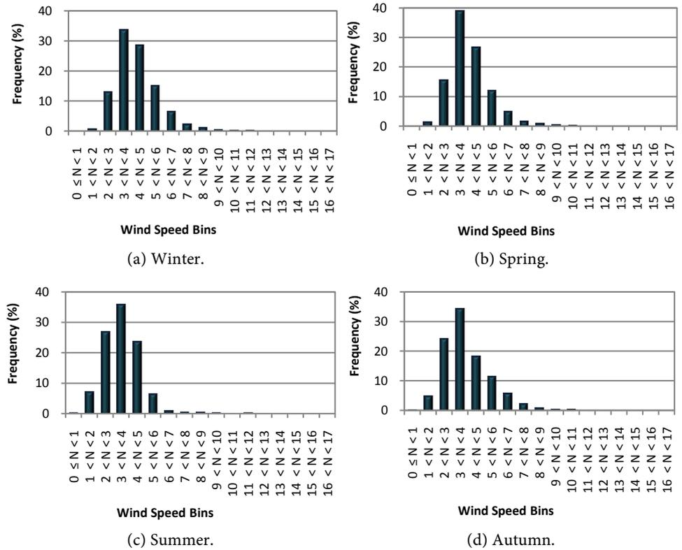
**Figure 10.** Seasonal percent frequency distribution of mean wind speed at 50 m above the ground level at different bins (Group III).
