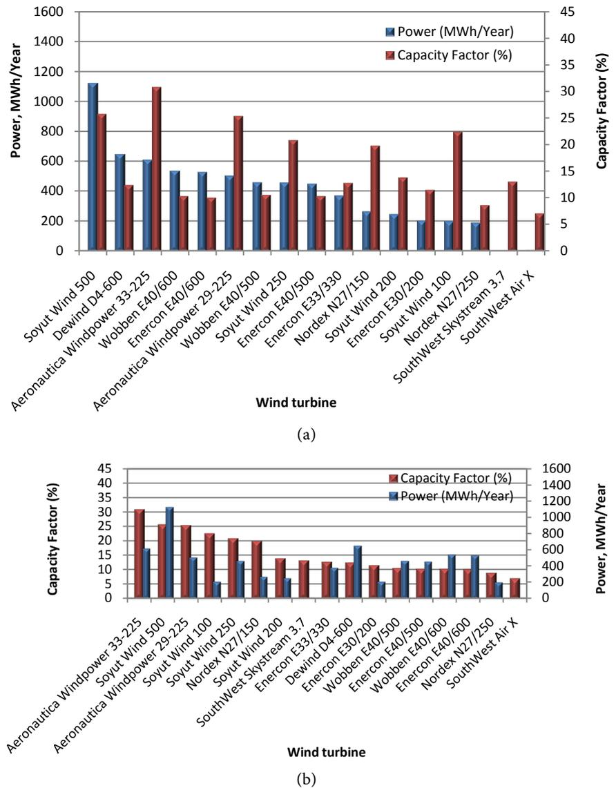
Figure 15. Annual power output and capacity factor from different machines at group III.
