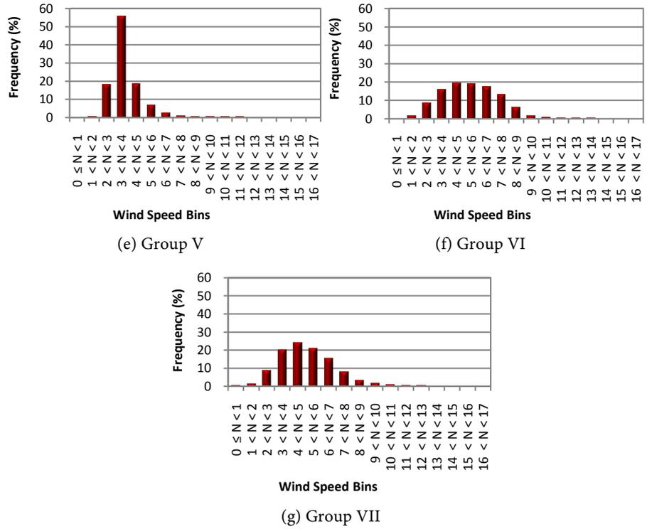
**Figure 9.** Annual percent frequency distribution of mean wind speed at 50 m above the ground level for the seven groups at different bins.
