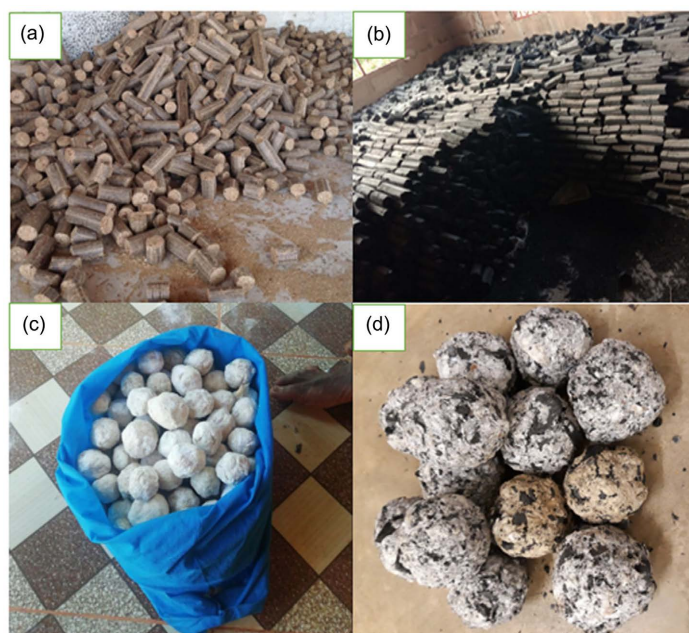
Figure 3. Briquettes obtained from stakeholders during field visit: (a) Non-carbonised stick; (b) carbonised hexagonal; (c) Non-carbonised spherical; (d) Spherical waste papers.
