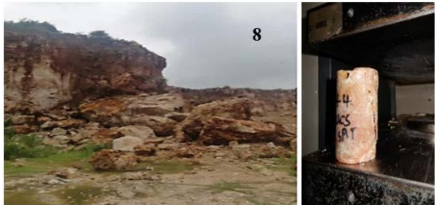
Figure 13. Litho8: Rock mass is blocky. UCS = 23.49, n = 5.31\% , GSI = 28.
