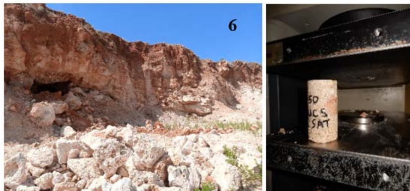
Figure 11. Litho6: Broken rock, clayey, UCS = 12.59 MPa, GSI = 18, n = 15.25\% .
