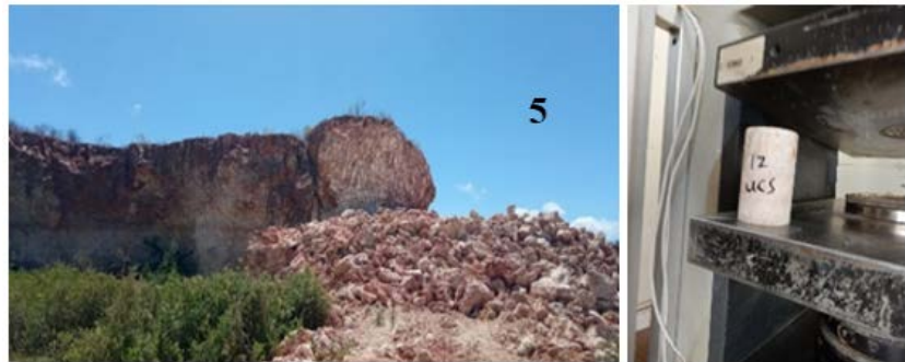
Figure 10. Litho5: Rock mass is blocky. UCS = 36.06 MPa, n = 5.4\% , GSI = 30.
