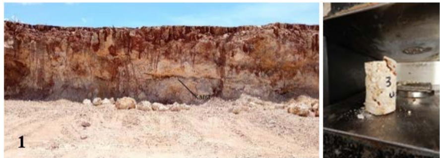
Figure 6. Litho1: Rock mass is poorly interlocked, pores and fissures filled with soil. UCS = 17.43 MPa, n = 11.82\% , GSI = 19.
