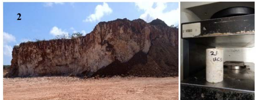
Figure 7. Litho2: Rock mass is blocky. UCS = 17.64 MPa, n = 1.56\% , GSI = 2.
