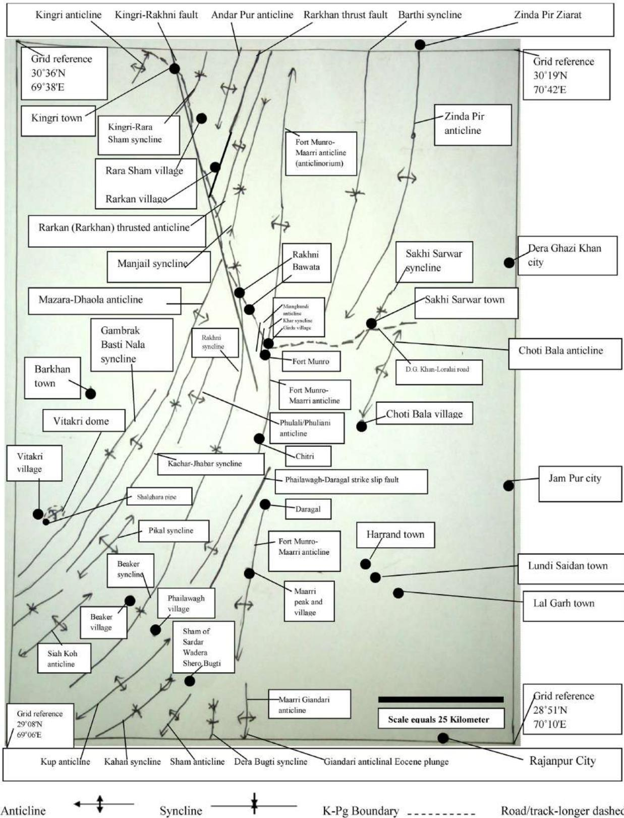
**Figure 6.** Structural major folds (anticlines and synclines) and faults of eastern Mari Bugti hills of Balochistan Province, Fort Munro-Maarri and Zinda Pir anticlines of eastern Sulaiman arc and Sulaiman foldbelt, South Punjab, Pakistan. For legend and symbols, see **Figure 3**.
