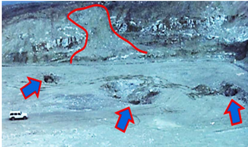
Figure 3. A karstified site, 15 km southeast of Mosul Dam, note the karstified gypsum beds (white color) and their total absence in the limited area by the red line (due to dissolution), and the developed sinkholes in the ground (After [8]).
