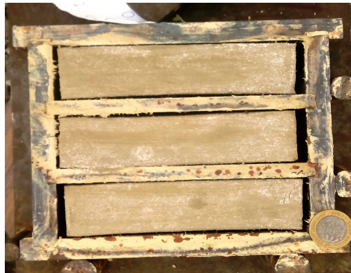
Figure 3. A sample of adhesive mortar.
