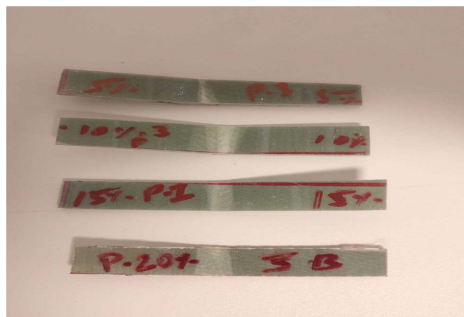
Figure 5. Flexural tested polyester samples (SiC).
