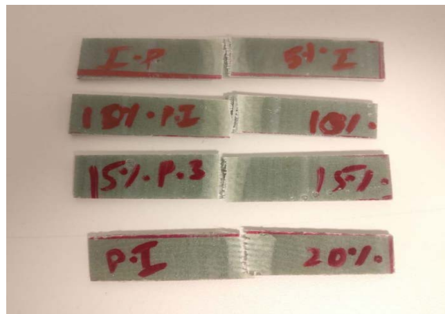
Figure 7. Impact tested polyester samples (SiC).
