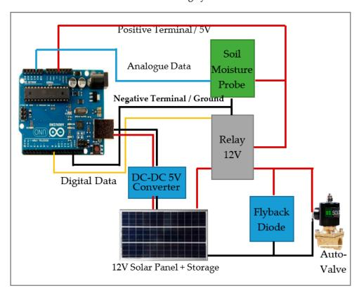
**Figure 8.** The proposed auto-watering system based mathematical model; red line is positive terminal; black line is ground; yellow line is digital data; blue is analogue data.
