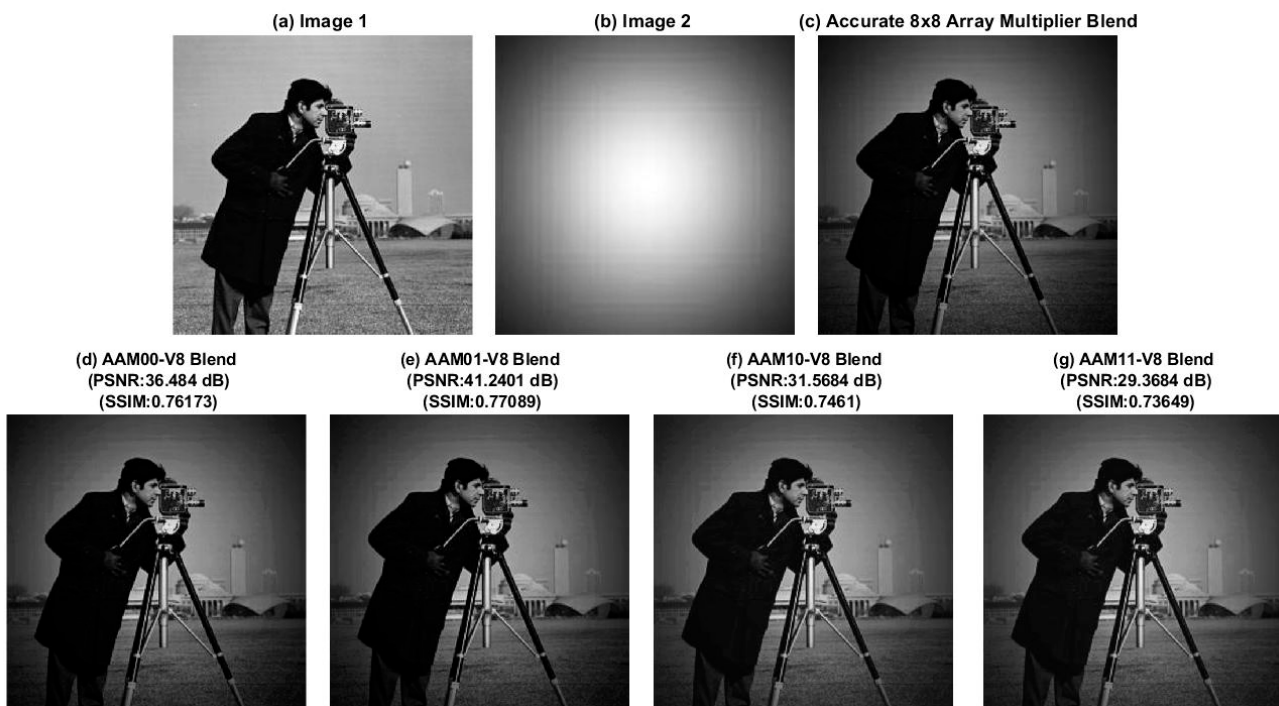
Figure 12. Blending of 'cameraman' and 'mask' images: (a) 'cameraman' image; (b) 'mask' image; (c) accurately blended images; (d) images blended using AAM00-V8; (e) images blended using AAM01-V8; (f) images blended using AAM10-V8; (g) images blended using AAM11-V8.
