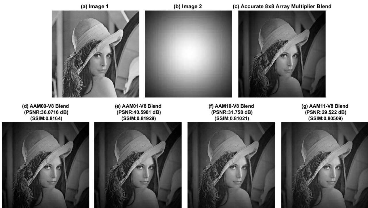
Figure 11. Blending of 'lena' and 'mask' images: (a) 'lena' image; (b) 'mask' image; (c) accurately blended images; (d) images blended using AAM00-V8; (e) images blended using AAM01-V8; (f) images blended using AAM10-V8; (g) images blended using AAM11-V8.
