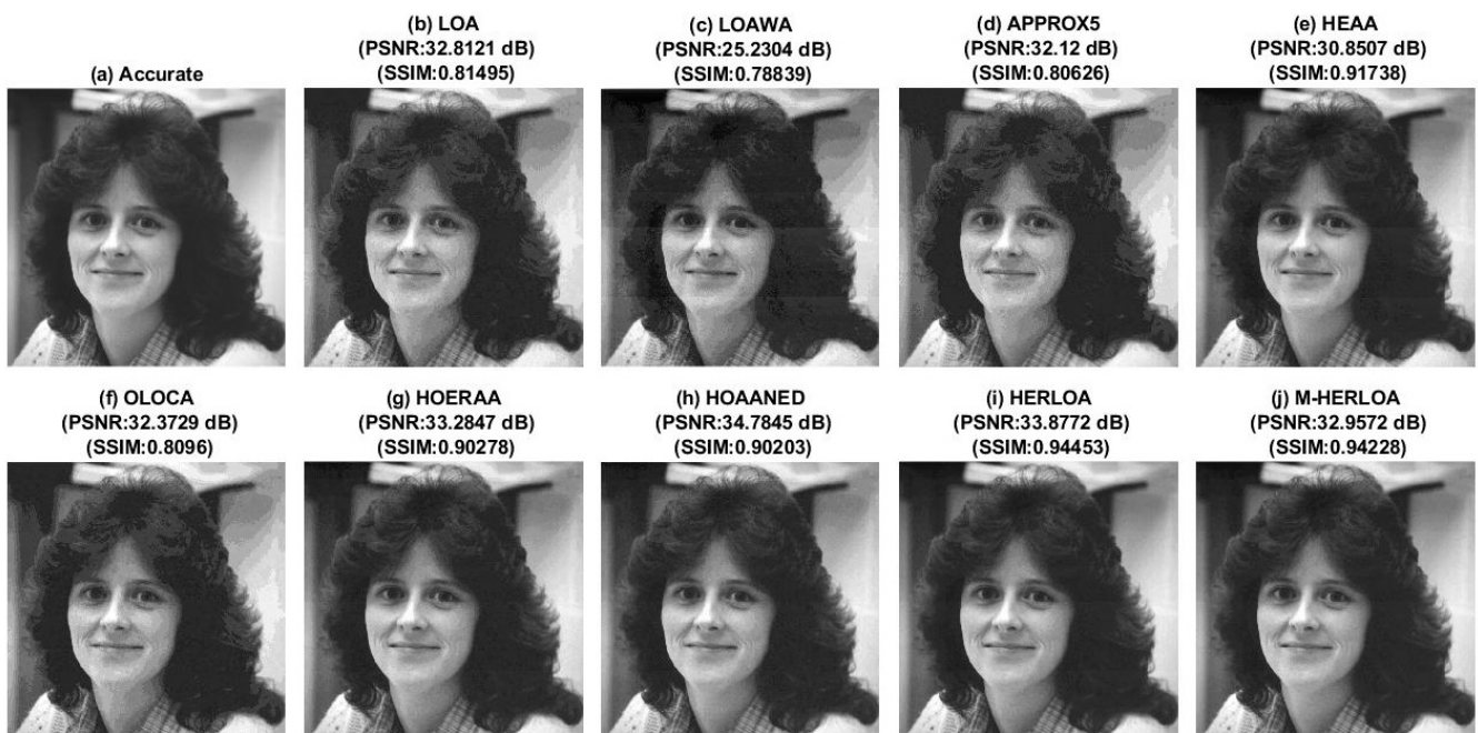
Figure 4. Image processing result for ‘woman with dark hair’ image obtained using accurate and approximate adders: (a) accurate adder; (b) LOA; (c) LOAWA; (d) APPROX5; (e) HEAA; (f) OLOCA; (g) HOERAA; (h) HOANED; (i) HERLOA; (j) M-HERLOA.
