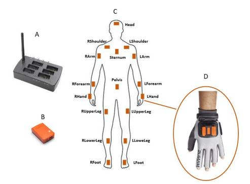
**Figure 3.** Experimental setup. (**A**) Hardware wireless station; (**B**) IMU motion tracker; (**C**) motion trackers positioning on the subject; (**D**) glove for finger tracking.
