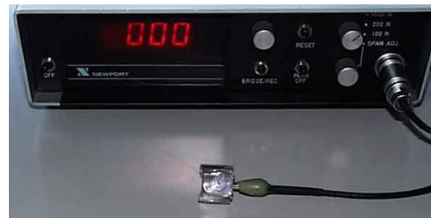
Figure 2. A photograph of the miniature pressure transducer used for the measurement of the bite force.
