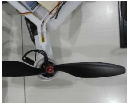
Figure 19. Monocoque Quadcopter structure with strain gauge.
