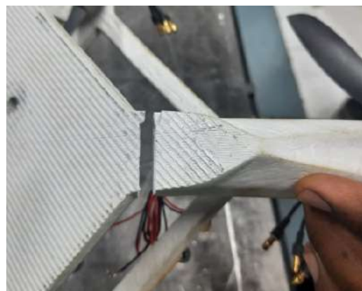
Figure 17. Failure at first natural frequency.
