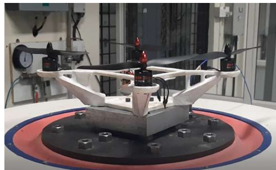
Figure 15. Quadcopter structure fixed to the shaker.
