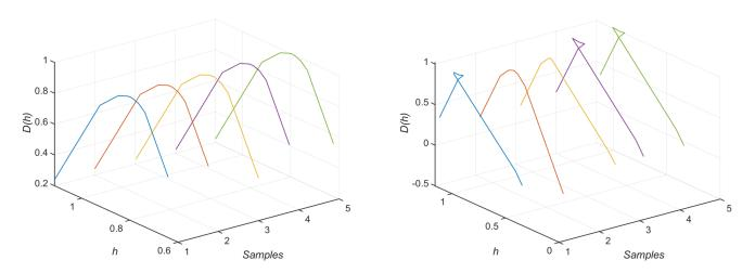
**Figure 5.** WLM D(h) signatures of: (**left**) normal traces, (**right**) abnormal traces.
