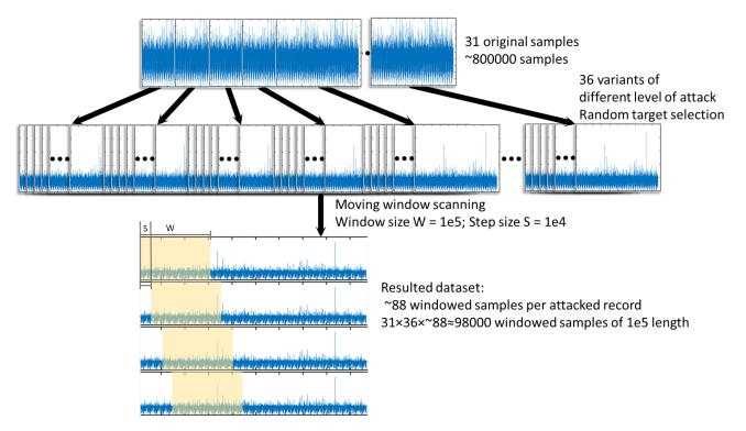
**Figure 4.** The process of dataset generation.
