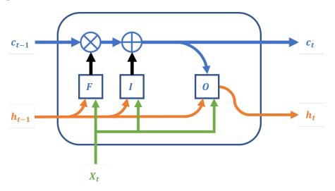
Figure 2. A simplified LSTM unit.
