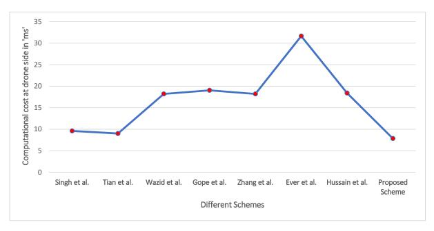
Figure 3. Computational cost at drone side for different schemes.
