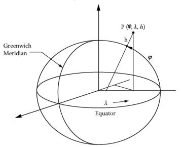
Figure 2. Three coordinate system representation.
