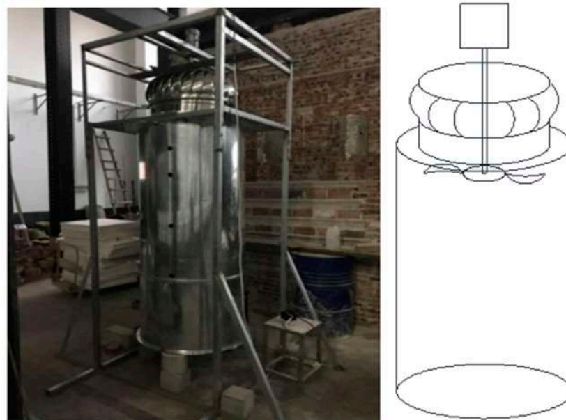
Figure 7. Performance optimization platform of a QM-600 swirl natural ventilator.
