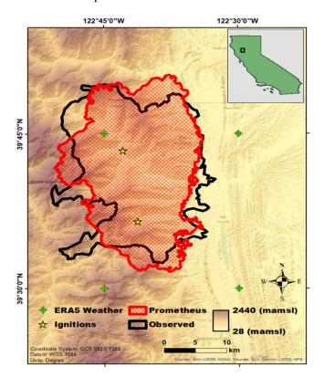
**Figure 2.** Observed (52,281 ha) and simulated (52,245 ha) Doe Fire perimeter on 22 August, after 96 h of explosive growth. ERA5 weather stream locations are marked with green locators.
