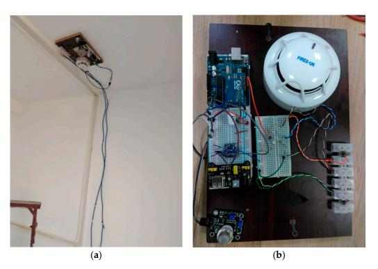
**Figure 2.** Hardware Deployment setup for Experiments: (**a**) setup physically situated in the middle of the laboratory room; (**b**) experimental setup showing sensors connected to the microcontroller motherboard and the LoRa Node wireless system connecting it to the cloud.
