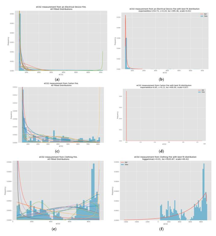
**Figure 7.** All the fitted distributions for the eCO<sub>2</sub> measurement for each fire source, namely, electrical device/clothing, charcoal/clothing, and charcoal/cardboard (**a**–**f**).
