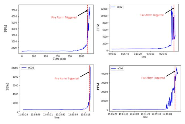
Figure 5. The eCO<sub>2</sub> reading measurements for four different experiments of electric fires.
