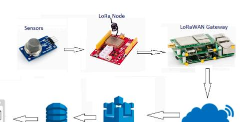
Figure 3. Communication Architecture for the experimental setup.
