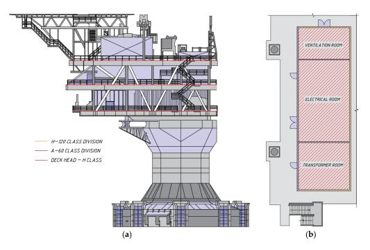
**Figure 2.** (a) Offshore platform with deck location. (b) Fragment of the section of the first deck with the arrangement of the bulkheads.
