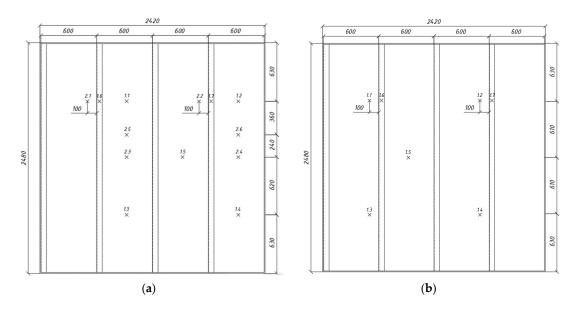
**Figure 3.** (a) Location of thermocouples on bulkhead H-120. (b) Location of thermocouples on bulkhead H-0.
