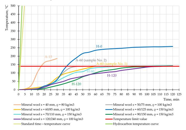
Figure 9. Temperature curves of experimental samples during fire tests.
