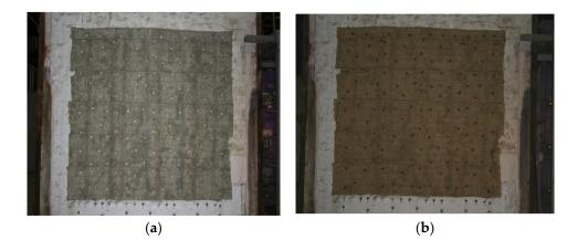
**Figure 4.** (a) Heated side of H-120 bulkhead before fire test. (b) Heated side of H-120 bulkhead after fire test.
