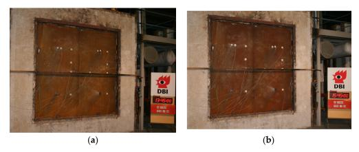
Figure 5. (a) H-120 bulkhead at the beginning of fire test. (b) H-120 bulkhead at the end of fire test.
