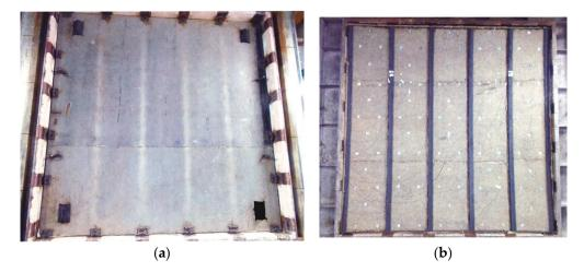
**Figure 7.** (a) Heated side of A-15 bulkhead at the end of the fire test. (b) Unheated side of A-15 bulkhead at the end of the fire test.
