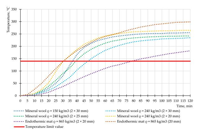
Figure 14. Variations of flame-retardant application for H-0 bulkhead.
