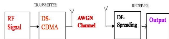
Fig 1: simple Block Diagram of DS-CDMA Transmitter and Receiver.
