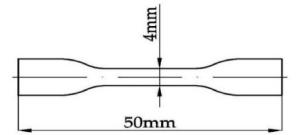
Figure 3. Samples used in tensile and shear experiments.
