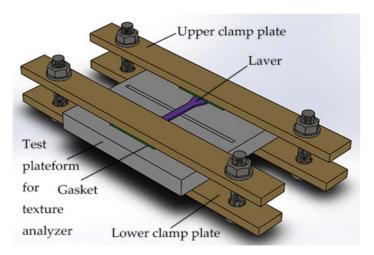
Figure 4. Clamp for the shear test.
