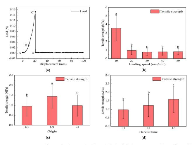
**Figure 7.** Tensile properties of laver: (a) the load–displacement curve of the tensile test of laver; (b) the effect of loading rate on tensile strength; (c) the effect of origin on tensile strength; (d) the effect of harvest time on tensile strength. The different lowercase letters indicate a significant difference between groups (p < 0.05), while same lowercase letters indicate no significant difference between groups (p > 0.05).
