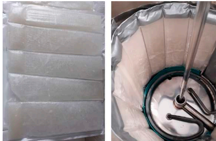
Figure 7. S34 PCM encapsulation, placed between the inner and outer tanks.
