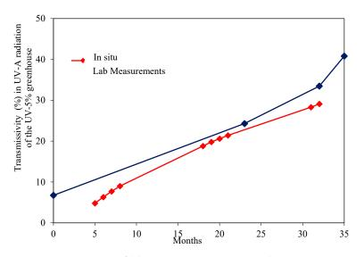
**Figure 4.** Comparison of laboratory measurements and in situ measurements for the UV-5% film in the UV-A region.
