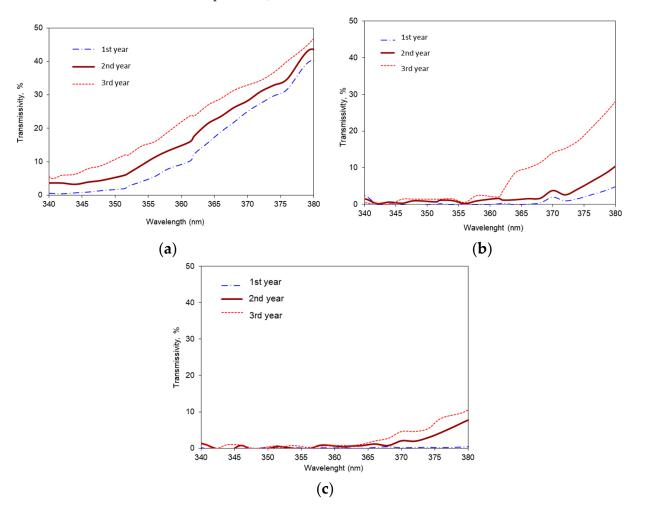
**Figure 2.** UV-A transmission coefficient evolution of the covering films for three years for: (**a**) UV-5% film; (**b**) UV-3% film; and (**c**) UV-0% film.
