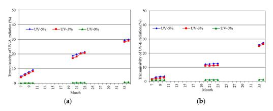
**Figure 3.** Monthly changes in covering material transmissivity for: (**a**) UV-A; and (**b**) UV-B radiation. The first measurement was taken seven months after the installation of the films.
