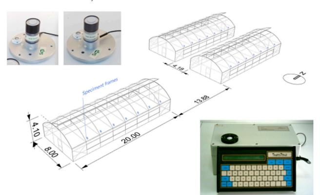
**Figure 1.** Layout and orientation of the experimental greenhouses. Specimen frames indicate places on the greenhouse roofs where samples of the material were cut off and their transmittance was evaluated. In situ measurements were performed with ultraviolet (UV)-B and UV-A radiation sensors (on the **top-left**), while a LI-COR-1800 instrument (**bottom-right**) was used in the laboratory measurements.
