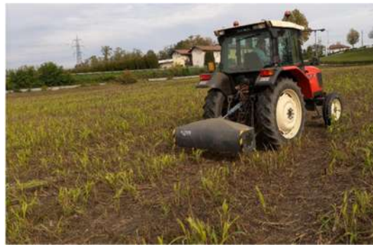
Figure 13. The SoilXplorer sensor rear-mounted on a tractor.
