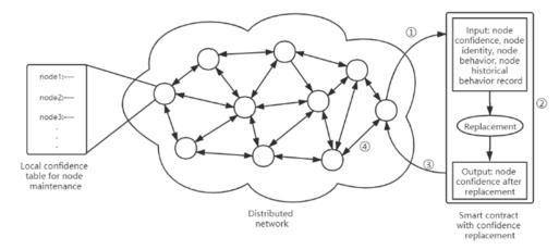
Figure 2. Reputation replacement based on smart contract.
