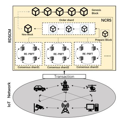
Figure 1. RDSCM applied in IoT network.
