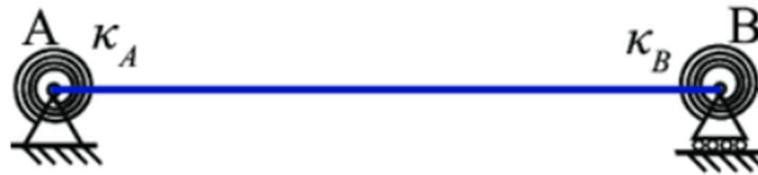
Figure 8. Simplified model that accounts for the rigidity of transverse stiffeners.
