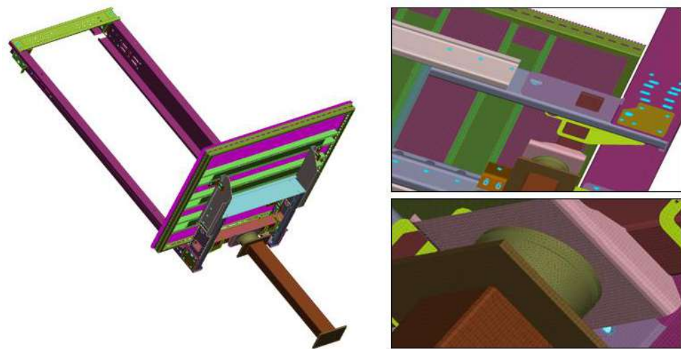
Figure 12. New-design elevator chassis FE model.
