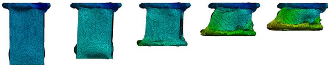
Figure 9. FE analysis of deformation process for the novel cell under axial load.
