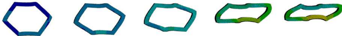
Figure 22. FE analysis of deformation process for the standard hexagonal cell under lateral load.
