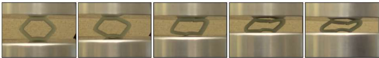
Figure 21. Experimental compression test of standard hexagonal cell under lateral load.
