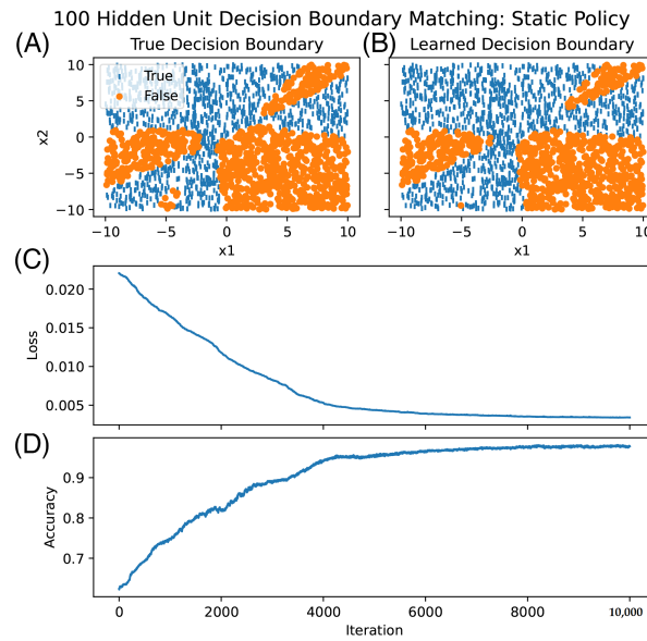
Figure 2. Static synaptic policy applied to 2D decision-boundary-matching task. The ground-truth decision boundary is shown in (A) while the learned decision boundary is in (B). Loss and accuracy scores per training iteration are shown in (C,D), respectively. Exploration probability \epsilon is set to 25%, synaptic learning rate \alpha_s = 0.001 , and future reward discount \gamma = 0.9 . tanh activation functions were used in both the trained and target networks. Final accuracy is 97.7%, while final mean Euclidean loss across the dataset is 0.003411.
